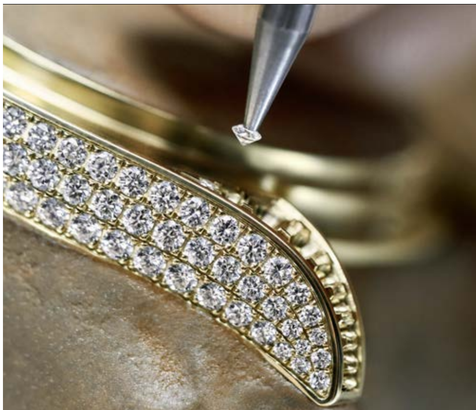
Setting diamonds into the watch case of the Oyster Perpetual Lady-Datejust
