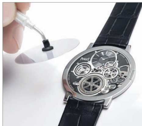
Placing the 0.2 mm sapphire crystal on the timepiece
