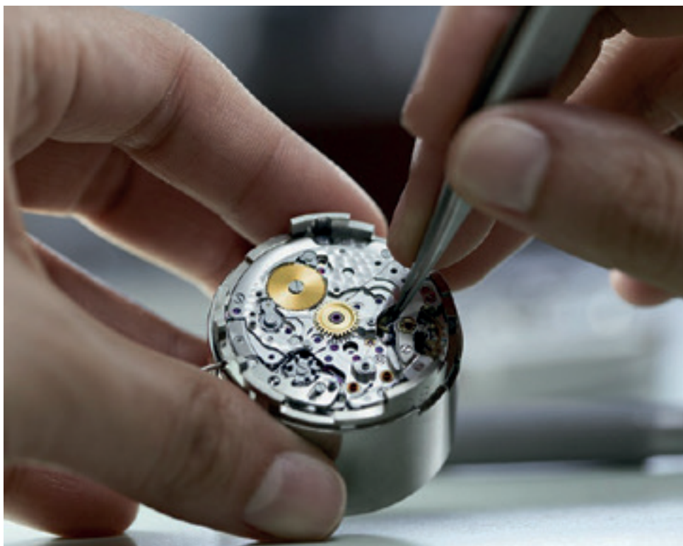
A Rolex watchmaker closely examines each individual component of the movement and identifies which components require replacement
